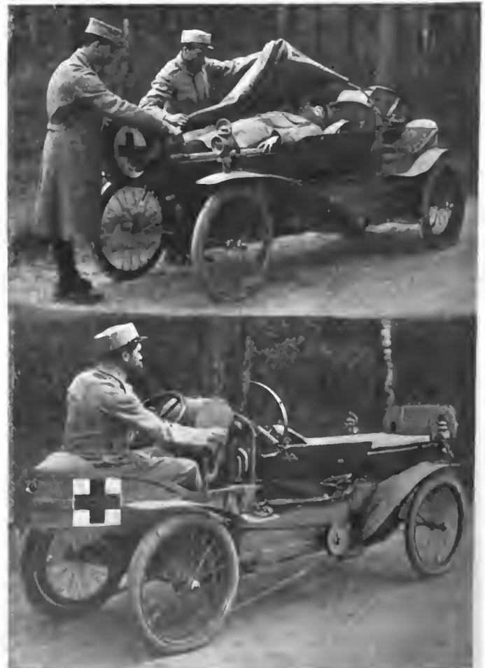
Above—Bringing in a wounded soldier on a cyclecar ambulance Below—Showing control and driver's seat. Note belt drive
